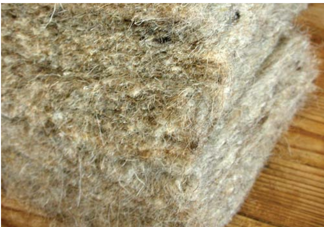
Sheep's wool makes ideal insulation material
